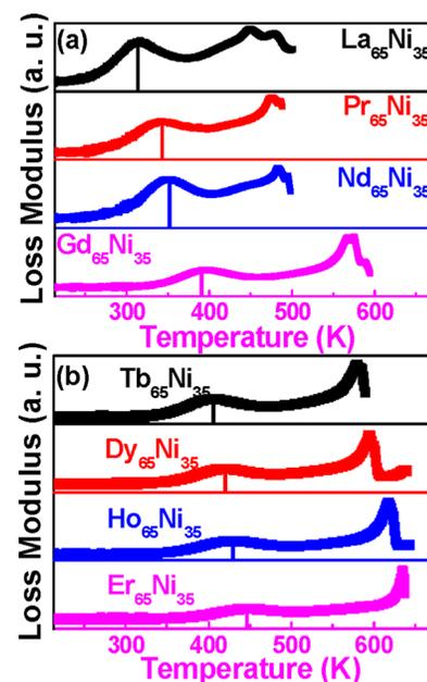
FIG. 2. Temperature dependence of the loss modulus  $G''$  for the  $\text{RE}_{65}\text{Ni}_{35}$  MGs, where RE represents (a) La, Pr, Nd, Gd and (b) Tb, Dy, Ho, Er. The line shows the position of the peak temperature of  $\beta$ -relaxation.
