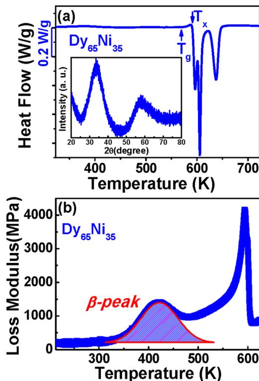
FIG. 1. (a) DSC traces of typical  $\text{Dy}_{65}\text{Ni}_{35}$  MG ribbon. The arrows designate the  $T_g$  and  $T_x$ . The inset shows XRD pattern of the MG. (b) Temperature dependence of the loss modulus  $G''$  for the  $\text{Dy}_{65}\text{Ni}_{35}$  MG. The shaded area represents the  $\beta$ -relaxation.
