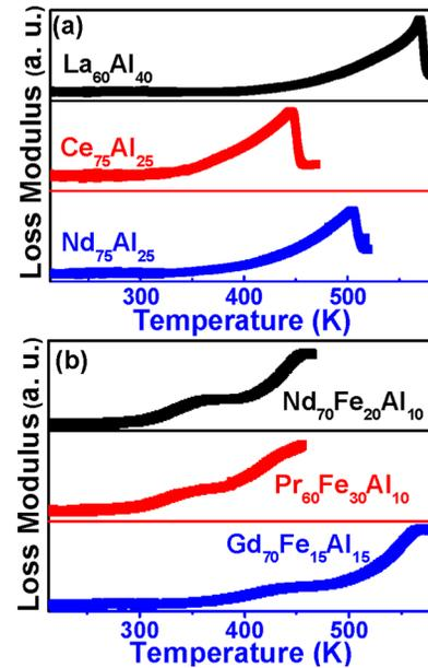
FIG. 4. (a) Temperature dependence of the loss modulus  $G''$  for the (a) RE-Al MGs, where RE represents La, Ce, and Nd, and (b) RE-Fe-Al MGs, where RE represents Nd, Pr, and Gd.
