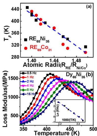
FIG. 3. (a) Relationship between the peak temperature of  $\beta$ -relaxation  $T_\beta$  and the relative atomic radii ratio between RE and Ni/Co. The error is of the order of the symbol size. (b) Temperature dependence of  $\beta$ -relaxation measured with frequencies of 0.5, 1, 2, 4, 8, and 16 Hz. The inset shows the plot of  $\ln f$  vs.  $1000/T_{\beta,peak}$ . The activation energy of  $\beta$ -relaxation  $E_\beta$  can be determined from the plot.
