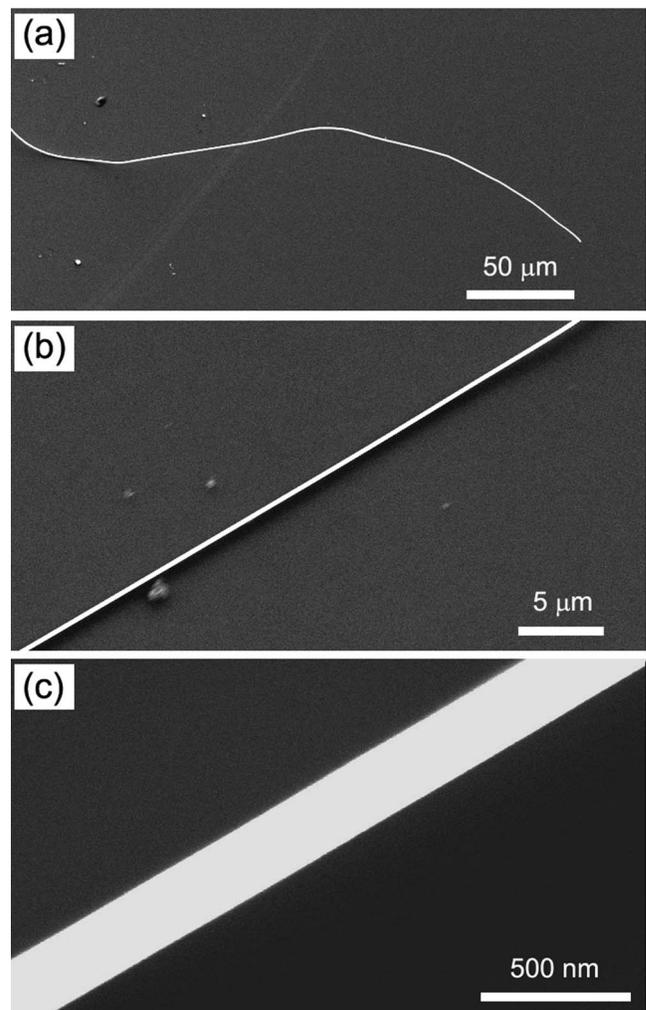
FIG. 4. SEM images of MGFs. (a) and (b) SEM picture of micro-scale  $\text{Pd}_{40}\text{Cu}_{30}\text{Ni}_{10}\text{P}_{20}$  MGFs. (c) SEM picture of nano-scale  $\text{Pd}_{40}\text{Cu}_{30}\text{Ni}_{10}\text{P}_{20}$  MGFs.
