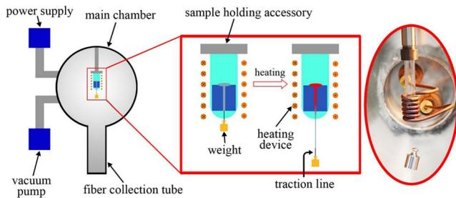
FIG. 1. General layout of metallic glassy fiber fabrication machine (left) and the schematic illustration for the principal of the supercooled liquid extraction method (right).
