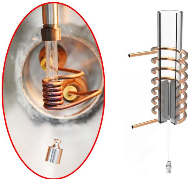
FIG. 2. The detail of the SLEM assembly (right) and its photo (left): A small low carbon steel cylinder, of which diameter and length is, respectively, 12.3 mm and 40 mm. There is a hole in the steel cylinder and the diameter of the hole in the low carbon steel cylinder is larger than that of the glassy rods. The MG rod is placed in the center of the hole, and then the rod together with the small cylinder is placed in a quartz glass tube.
