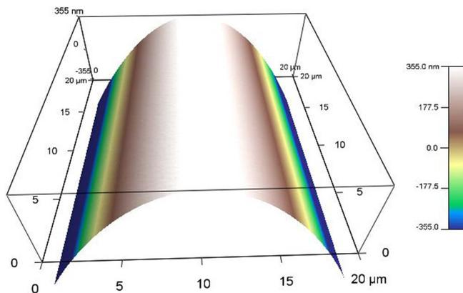
FIG. 6. The atomic force microscopy (AFM) picture of surface smoothness of  $\text{Pd}_{40}\text{Cu}_{30}\text{Ni}_{10}\text{P}_{20}$  MGFs.
