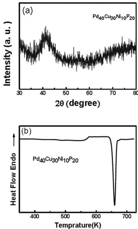
FIG. 5. (a) The x-ray diffraction spectrum from the  $\text{Pd}_{40}\text{Cu}_{30}\text{Ni}_{10}\text{P}_{20}$  MGFs. (b) The DSC result which shows that the fiber has a distinctive glass transition temperature.
