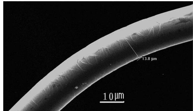
FIG. 8. SEM picture of bended  $\text{Pd}_{40}\text{Cu}_{30}\text{Ni}_{10}\text{P}_{20}$  MGFs.
