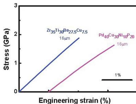
FIG. 7. The tensile stress-strain curves for  $\text{Zr}_{35}\text{Ti}_{30}\text{Be}_{27.5}\text{Cu}_{7.5}$  MGFs and  $\text{Pd}_{40}\text{Cu}_{30}\text{Ni}_{10}\text{P}_{20}$  MGFs at a strain rate of  $2 \times 10^{-4} \text{ s}^{-1}$  SEM picture of bended  $\text{Pd}_{40}\text{Cu}_{30}\text{Ni}_{10}\text{P}_{20}$  MGFs.
