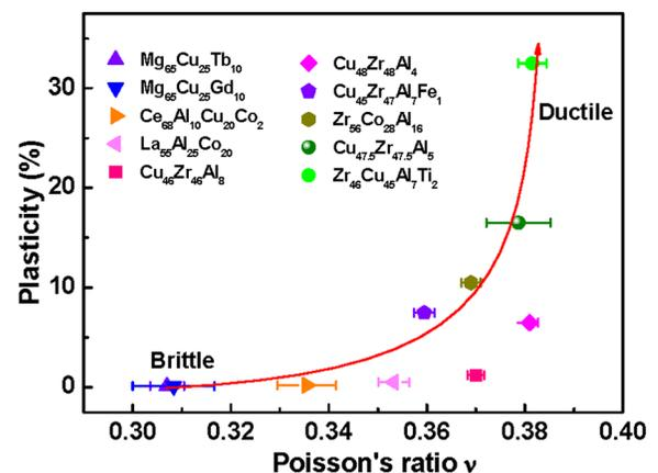
FIG. 1. The correlation of room-temperature comprehensive plasticity and Poisson's ratio for ten as-cast MGs with diverse compositions and properties.
