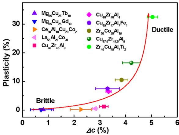
FIG. 2. The correlation of room-temperature comprehensive plasticity and the relative change of the concentration of the flow units  $\Delta c$  for ten as-cast MGs.
