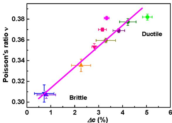
FIG. 3. Poisson's ratio vs. the relative change of the concentration of the flow unit  $\Delta c$  for various MGs in as-cast state. The MGs with larger density change of flow units show larger Poisson's ratio and better plasticity.
