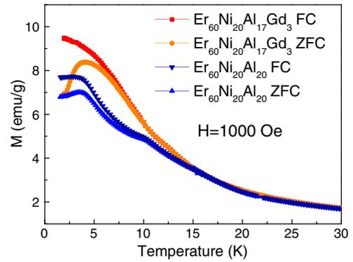
Fig. 5. Temperature dependence of the ZFC and FC magnetization under a magnetic field of 1000 Oe for  $\text{Er}_{60}\text{Ni}_{20}\text{Al}_{20}$  and  $\text{Er}_{60}\text{Ni}_{20}\text{Al}_{17}\text{Gd}_3$  alloys.
