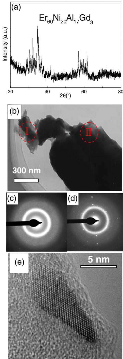
**Fig. 1.** Microstructure of  $\text{Er}_{60}\text{Ni}_{20}\text{Al}_{17}\text{Gd}_3$  alloy. (a) XRD pattern of the as-cast  $\text{Er}_{60}\text{Ni}_{20}\text{Al}_{17}\text{Gd}_3$  rods (diameter is 1 mm), (b) Bright-field TEM image of the alloy, (c) SAED pattern of part I showing in (b), (d) SAED pattern of part II showing in (b), (e) HRTEM image of part II showing in (b).
