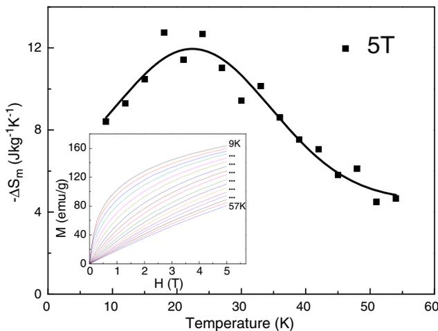
Fig. 4. The calculated magnetic entropy change from the Maxwell equation of the  $\text{Er}_{60}\text{Ni}_{20}\text{Al}_{17}\text{Gd}_3$  alloy under 5 T. The insert shows the magnetization isotherms of the  $\text{Er}_{60}\text{Ni}_{20}\text{Al}_{17}\text{Gd}_3$  alloy.
