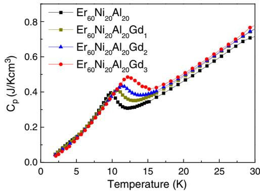
Fig. 3. Temperature dependence of the volumetric specific heats of the  $\text{Er}_{60}\text{Ni}_{20}\text{Al}_{20-x}\text{Gd}_x$  ( $x=0, 1, 2, 3$ ) alloys.
