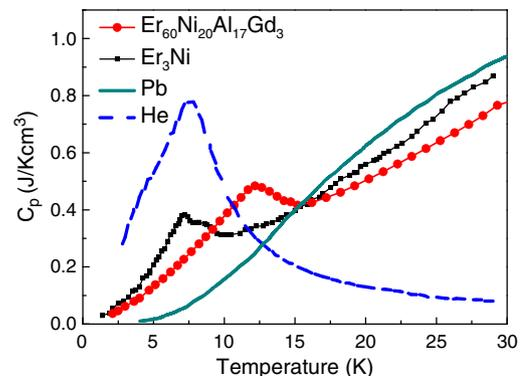
**Fig. 2.** The comparison of temperature dependence of the volumetric specific heats of He, Pb,  $\text{Er}_3\text{Ni}$  and  $\text{Er}_{60}\text{Ni}_{20}\text{Al}_{17}\text{Gd}_3$ .
