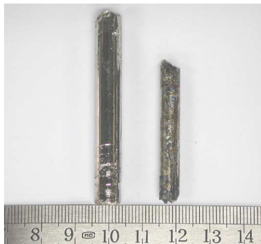
Fig. 2. A camera photo of \text{Fe}_{44}\text{Mn}_{11}\text{Cr}_{10}\text{Mo}_{12}\text{C}_{15}\text{B}_6\text{Ho}_2 SAS samples prepared in argon (left) and air (right) atmospheres.
