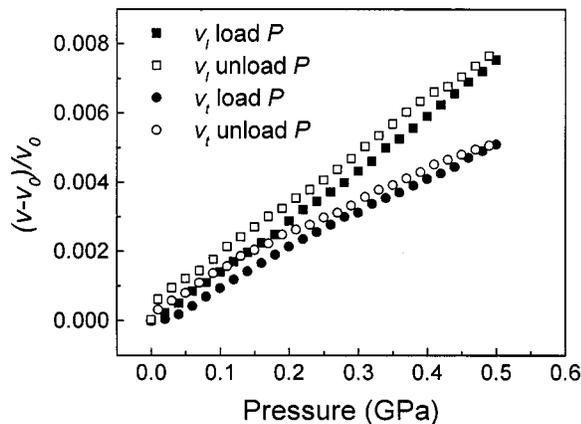
FIG. 1. Pressure dependence of the longitudinal and transverse acoustic velocities,  $v_l$  and  $v_t$ , of the Pd<sub>39</sub>Ni<sub>10</sub>Cu<sub>30</sub>P<sub>21</sub> BMG.  $v_0$  is the velocity at ambient pressure  $P_0$ .
