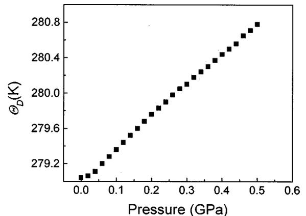
FIG. 3. Debye temperature of the Pd<sub>39</sub>Ni<sub>10</sub>Cu<sub>30</sub>P<sub>21</sub> BMG as a function of pressure.
