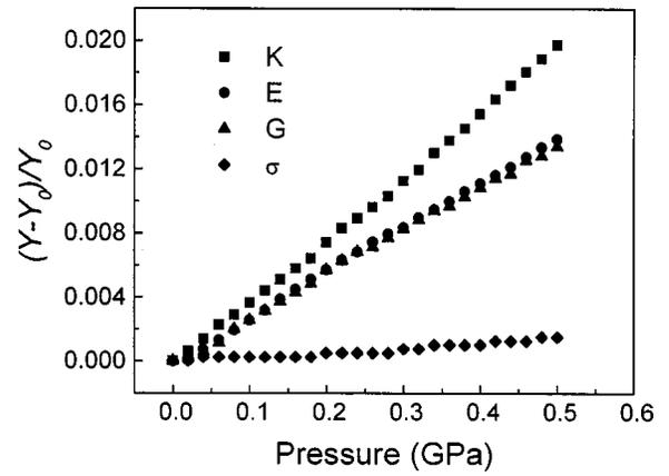
FIG. 2. Variation of the elastic constants of the Pd<sub>39</sub>Ni<sub>10</sub>Cu<sub>30</sub>P<sub>21</sub> BMG with pressure ( $Y=K,E,G,\sigma$ ).  $K$ ,  $E$ ,  $G$ , and  $\sigma$  stand for bulk modulus, Young's modulus, shear modulus, and Poisson's ratio.  $Y_0$  is the modulus at ambient pressure.
